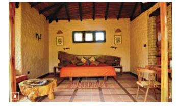
MATERIALS: WALLS Polygonal stone (main building) and brick with mud finish plaster. **FLOORING** Flagstone (main building) and terracotta tile (cottages). CEILING Terracotta tiles on wooden rafters with a waste wood false ceiling. **FURNITURE** Organic furniture with recycled unsawn wood and recycled sleeper wood. FURNISHINGS Bamboo chicks (window covering) and vegetable-dyed cotton.
